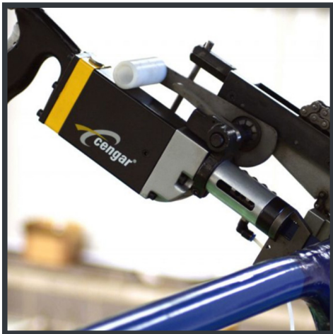
High Quality Steel Pipe up to 150mm dia and similar size sections.
